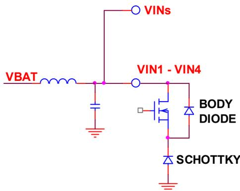
Figure 17. VINS pin connected directly to VIN1/2/3/4 pins
