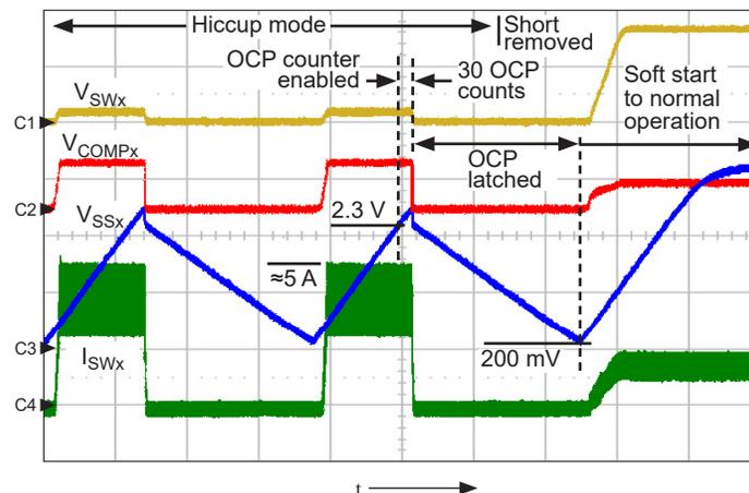
Figure 20. Hiccup mode and recovery to  $V_{SWx} = 3.3$  V at  $I_{SWx} = 1.6$  A; shows  $V_{SWx}$  (ch1, 2 V/div),  $V_{COMPx}$  (ch2, 2 V/div),  $V_{SSx}$  (ch3, 1 V/div),  $I_{SSSUx}$  (ch4, 2 A/div);  $t = 2$  ms/div
