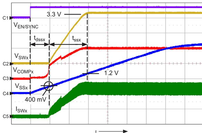
Figure 13. Normal startup to  $V_{SWx} = 3.3$  V at  $I_{SWx} = 1.6$  A load; shows  $V_{EN/SYNC}$  (ch1, 10 V/div.),  $V_{SWx}$  (ch2, 1 V/div.),  $V_{COMP}$  (ch3, 500 mV/div.),  $V_{SSx}$  (ch4, 1 V/div.),  $V_{SWx}$  (ch5, 1 A/div.),  $t = 500$   $\mu$ s/div.
