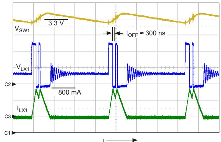
Figure 12. SW1 PFM operation at  $V_{IN1} = 12$  V,  $V_{SW1} = 3.3$  V,  $V_{SW1} = 120$  mA load, LX1 turns on twice every 18  $\mu$ s to regulate  $V_{SW1}$ ; shows  $V_{SW1}$  (ch1, 100 mV/div.),  $V_{LX1}$  (ch2, 5 V/div.),  $I_{LX1}$  (ch3, 500 mA/div.),  $t = 5$   $\mu$ s/div.
