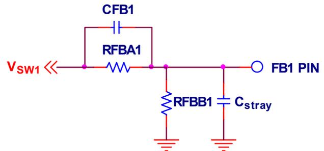
Figure 22. Addition of CFB1 to cancel stray capacitance
