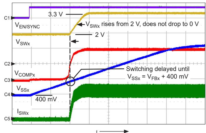
Figure 14. Pre-biased startup from  $V_{SWx} = 2$  V rising to 3.3 V at  $I_{SWx} = 1.6$  A load; shows  $V_{EN/SYNC}$  (ch1, 10 V/div.),  $V_{SWx}$  (ch2, 1 V/div.),  $V_{COMP}$  (ch3, 500 mV/div.),  $V_{SSx}$  (ch4, 1 V/div.),  $V_{SWx}$  (ch5, 1 A/div.),  $t = 500$   $\mu$ s/div.
