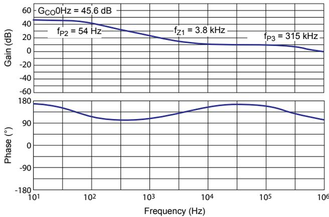
Figure 26. Compensated error amplifier Bode plot (SW3)
