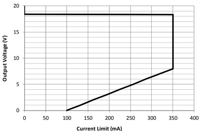
Figure 15. Typical DC current fold back versus V<sub>OUTx</sub> of S1 and S2
