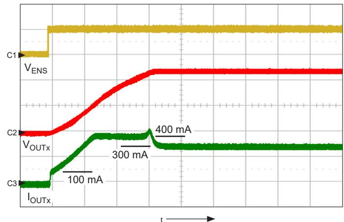
Figure 16. S1/S2 OUTx turning on with a load of 40 Ω and 22 μF; shows V<sub>ENS</sub> (ch1, 5 V/div.), V<sub>OUTx</sub> (ch2, 5 V/div.), I<sub>OUTx</sub> (ch3, 200 mA/div.), t = 500 μs/div.
