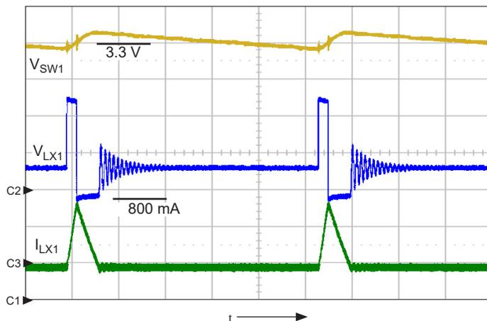
Figure 11. SW1 PFM operation at  $V_{IN1} = 12$  V,  $V_{SW1} = 3.3$  V,  $V_{SW1} = 50$  mA load, LX1 turns on once every 26  $\mu$ s to regulate  $V_{SW1}$ ; shows  $V_{SW1}$  (ch1, 100 mV/div.),  $V_{LX1}$  (ch2, 5 V/div.),  $I_{LX1}$  (ch3, 500 mA/div.),  $t = 5$   $\mu$ s/div.
