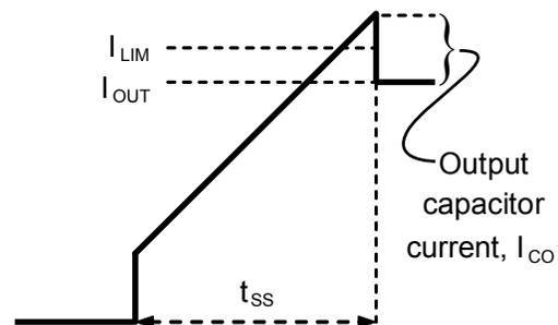
Figure 24. Output current ( $I_{CO}$ ) during startup
