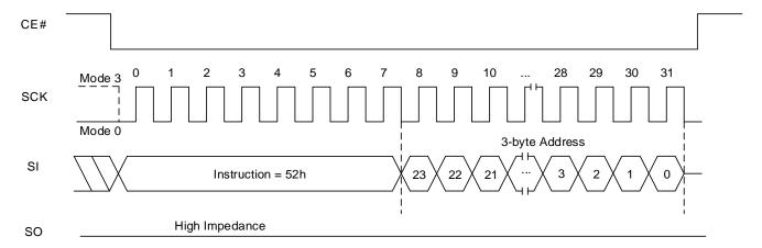
Figure 8.19 Block Erase (32K) Sequence In QPI Mode
