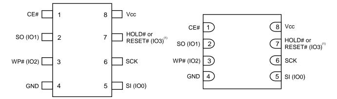
8-pin SOIC 208mil (Package: B) 8-pin SOIC 150mil (Package: N) 8-pin VVSOP 150mil (Package: V) 8-pin USON 2x3mm (Package: U) 8-pin USON 4x3mm (Package: T) 8-pin WSON 6x5mm (Package: K) 8-pin WSON 8x6mm (Package: L)
