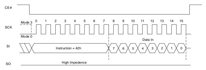
Figure 8.33 Write Function Register QPI Sequence In QPI Mode
