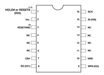
16-pin SOIC 300mil (Package: M)
