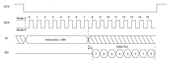
Figure 8.31 Read Function Register Sequence In QPI Mode
