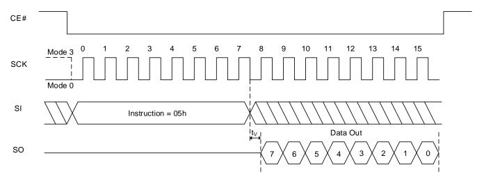
Figure 8.27 Read Status Register Sequence In QPI Mode
