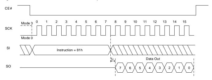
Figure 8.47 Read Extended Read Parameters Sequence In QPI Mode
