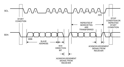
Figure 3. Data Transfer on I<sup>2</sup>C Serial Bus
