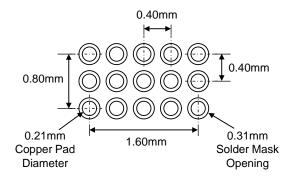
\* Dimensions are in millimeters.
