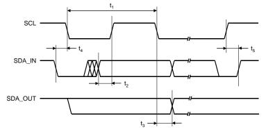
Figure 1. I<sup>2</sup>C Compatible Interface Timing
