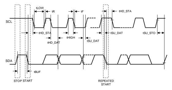
Figure 2. I<sup>2</sup>C Mode Timing Diagram
