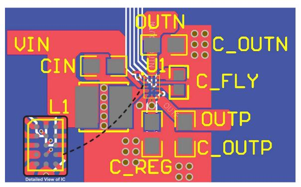
Figure 7. CSP Recommended PCB Layout
