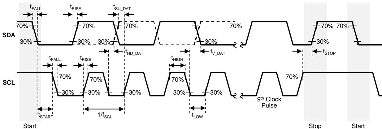
**Figure 1. I<sup>2</sup>C Compatible Interface Timing**
