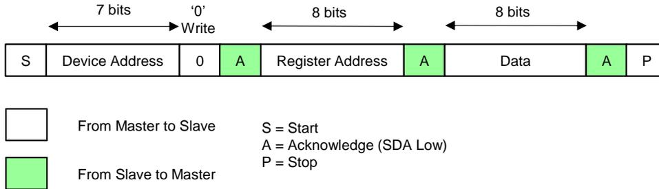
Figure 6. I<sup>2</sup>C Write Cycle
