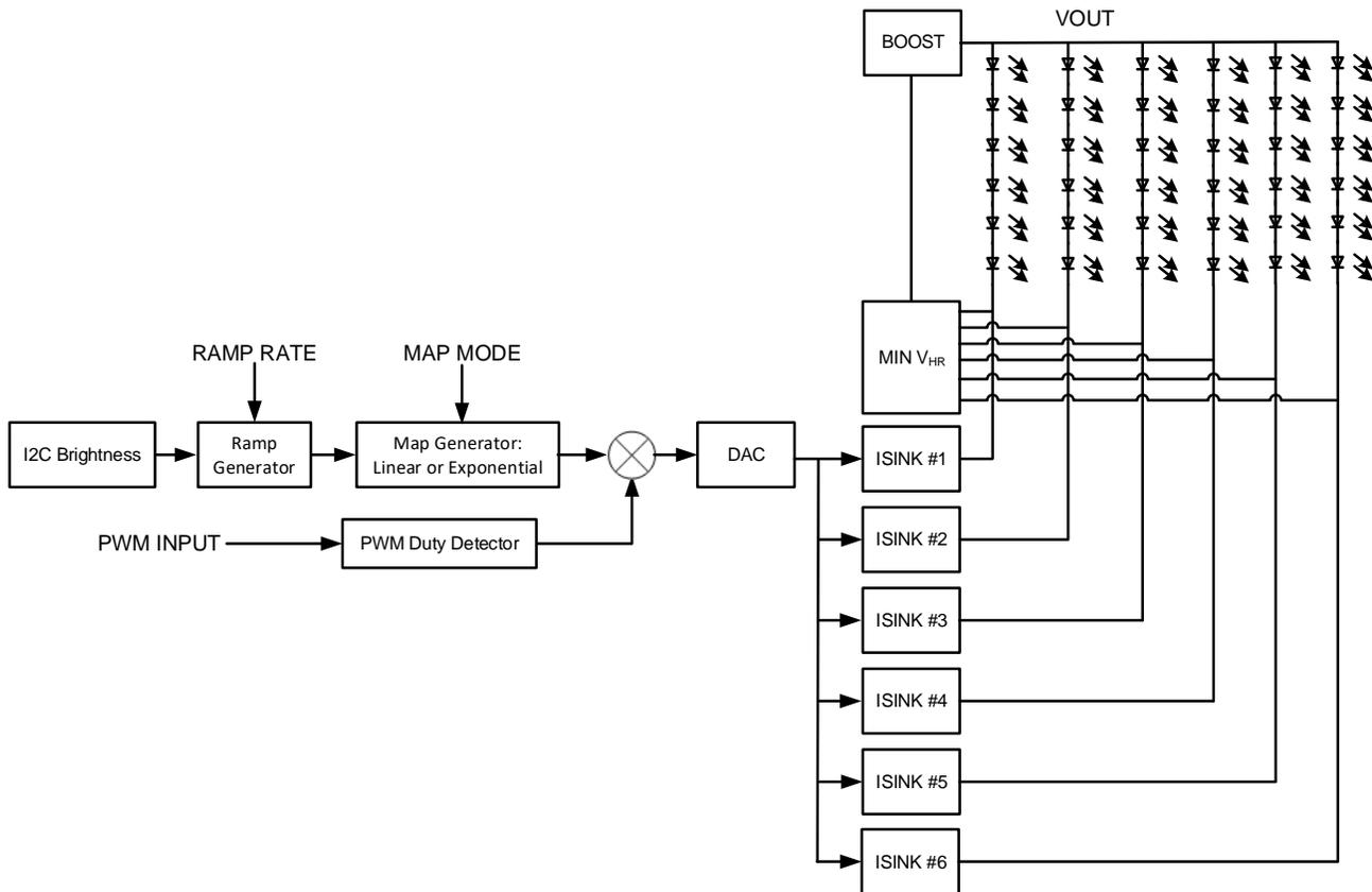
**Figure 4. I<sup>2</sup>C and PWM Dimming Scheme**
