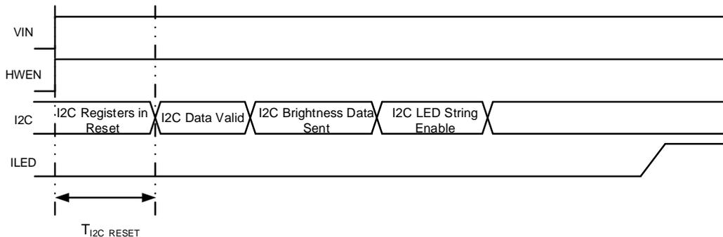
**Figure 2. Enable of KTZ8866 via I<sup>2</sup>C**
