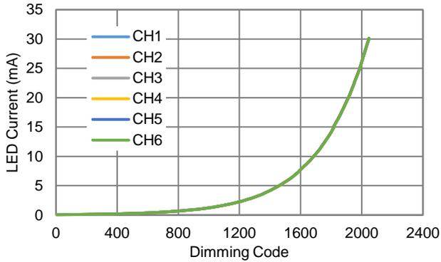
**LED Current vs. Current Ratio Code**
