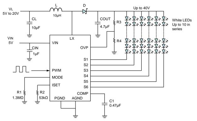
Figure 3. Inductor powered from a higher supply voltage
