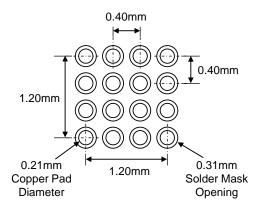
\* Dimensions are in millimeters.
