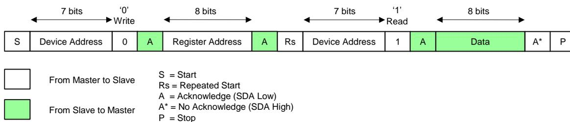
**Figure 7. I<sup>2</sup>C Read Cycle**
