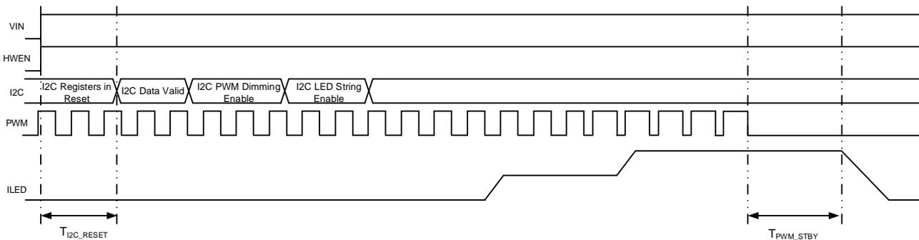
**Figure 3. Enable of KTZ8864A via PWM**
