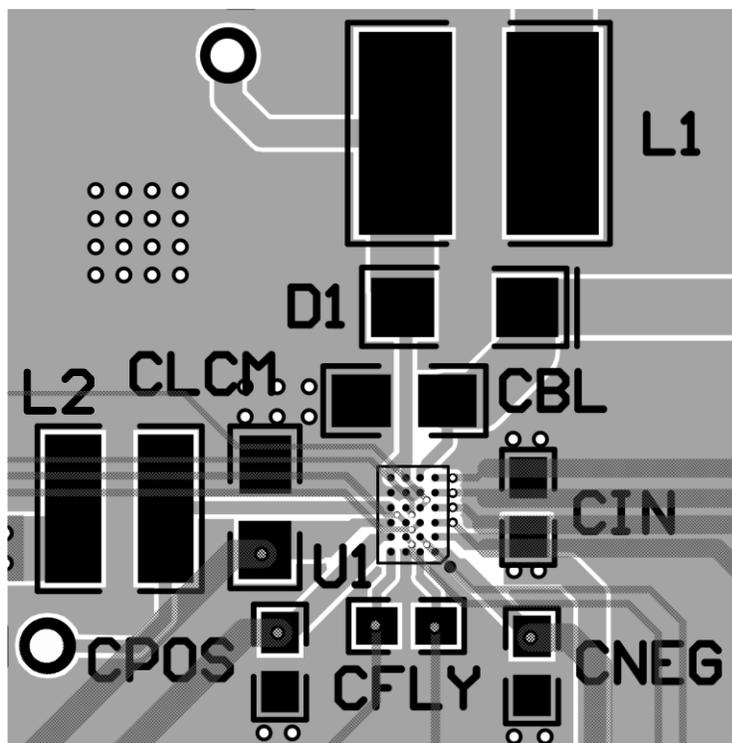
**Figure 8. Recommended PCB Layout**
