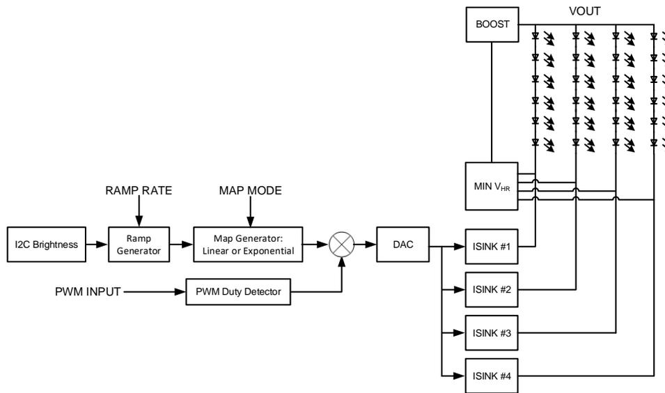
**Figure 4. I<sup>2</sup>C and PWM Dimming Scheme**
