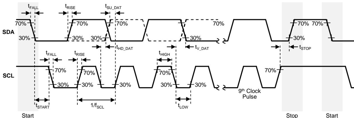
Figure 1. I<sup>2</sup>C Compatible Interface Timing
