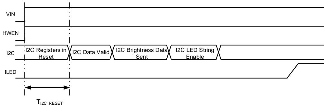
**Figure 2. Enable of KTZ8864A via I<sup>2</sup>C**
