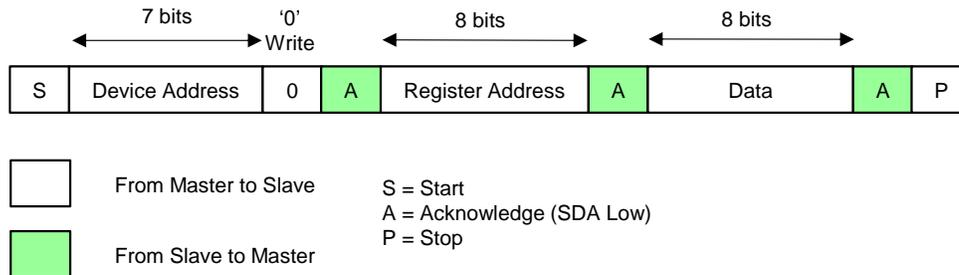
**Figure 6. I<sup>2</sup>C Write Cycle**
