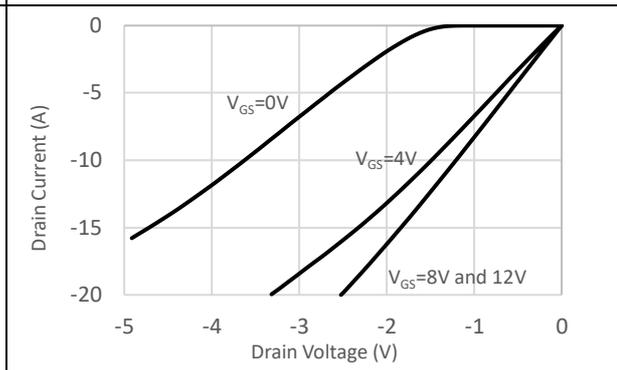
Figure 8. Reverse output characteristics at  $T_J = 150\text{ }^\circ\text{C}$ .
