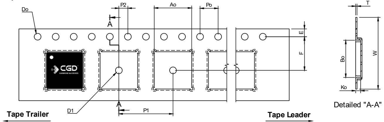
Tape Trailer - a minimum length of 160mm empty cavities sealed with cover tape.
