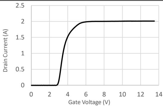
Figure 12. Transfer characteristics at  $V_{DS} = 0.1\text{ V}$ ,  $T_j = 25\text{ °C}$ .
