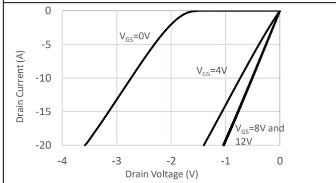
Figure 7. Reverse output characteristics at  $T_J = 25\text{ }^\circ\text{C}$ .
