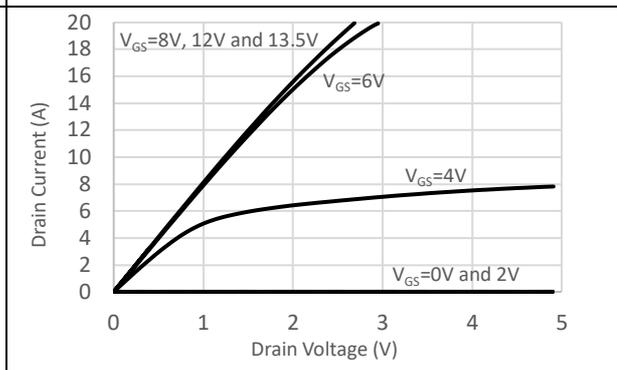
Figure 6. Forward output characteristic at  $T_J = 150\text{ }^\circ\text{C}$ .
