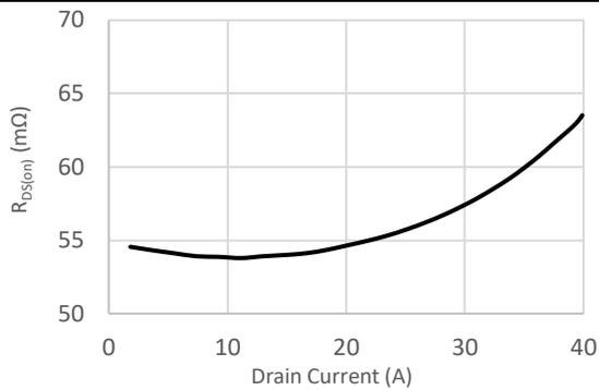
Figure 10. On-state resistance as a function of drain current at  $T_j = 25\text{ °C}$ .
