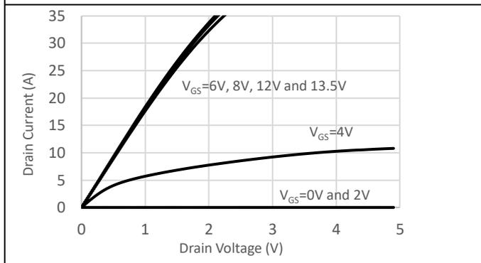
Figure 5. Forward output characteristics at  $T_J = 25\text{ }^\circ\text{C}$ .
