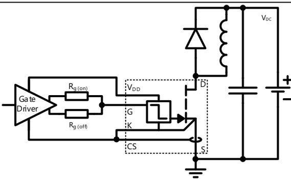
Figure 17. Inductive switching circuit.  $I_D = 10\text{ A}$ ,  $R_{g(on)} = 15\text{ }\Omega$ ,  $R_{g(off)} = 2\text{ }\Omega$ ,  $V_{DD} = 12\text{ V}$ ,  $V_{DC} = 400\text{ V}$ ,  $L = 125\text{ }\mu\text{H}$ , diode = IDH04G65C5.
