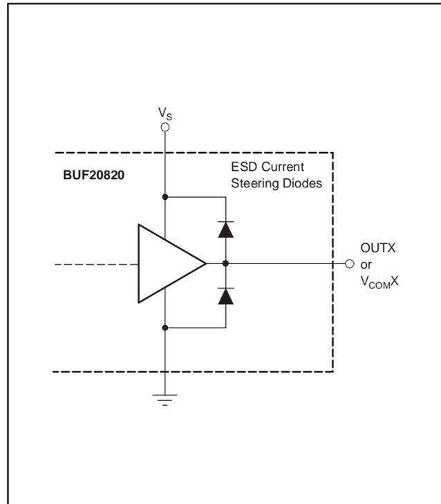
Figure 22. Output Pins ESD Protection Current-Steering Diodes
