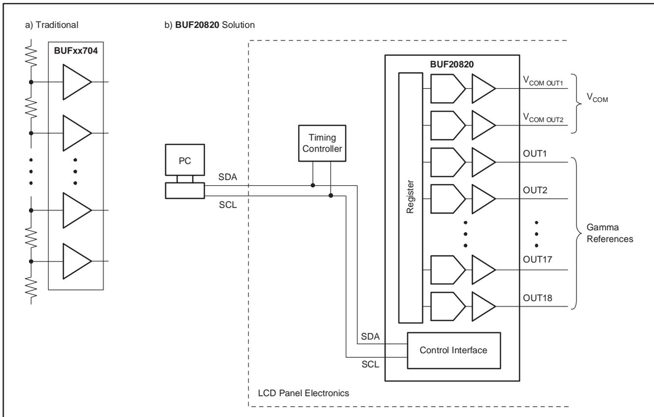
Figure 13. Replacement of the Traditional Gamma Buffer
