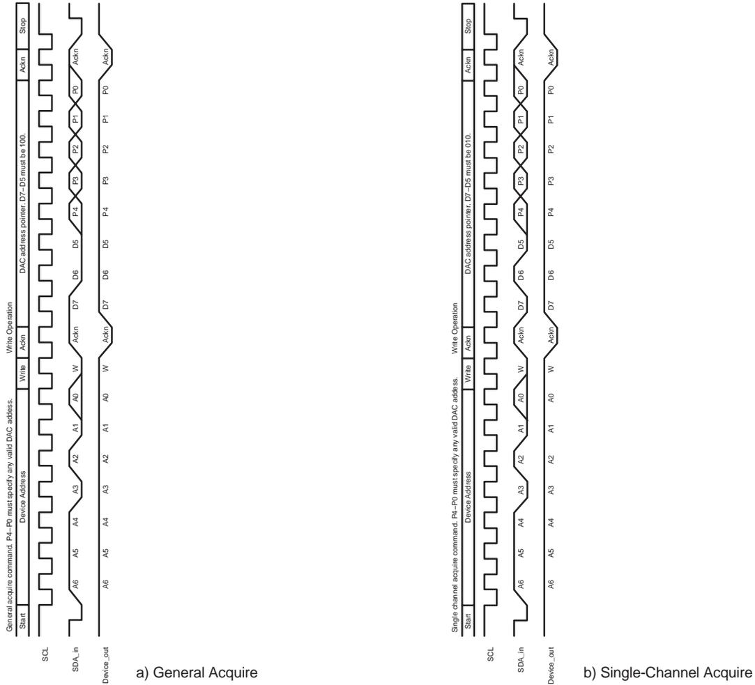
Figure 9. Timing Diagram for Acquire Operation
