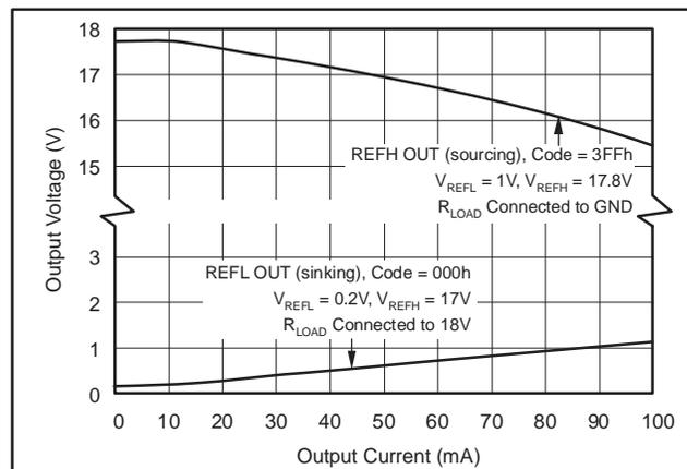
Figure 15. Reference Buffer Output Voltage vs Output Current
