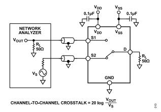
Figure 28. Channel-to-Channel Crosstalk
