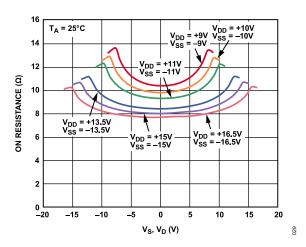
Figure 4. R<sub>ON</sub> as a Function of V<sub>D</sub> (V<sub>S</sub>), Dual Supply
