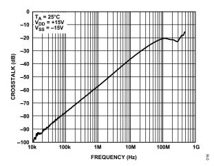
Figure 17. Crosstalk vs. Frequency, ±15 V Dual Supply
