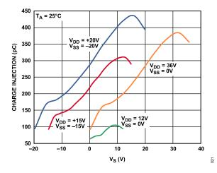
Figure 19. Charge Injection vs. Source Voltage
