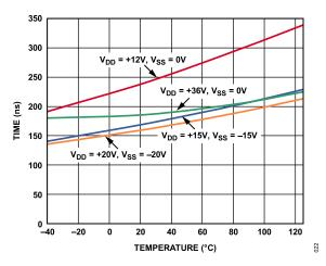
Figure 20. Transition Time vs. Temperature
