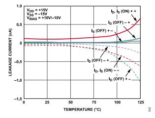
Figure 12. Leakage Currents vs. Temperature, ±15 V Dual Supply
