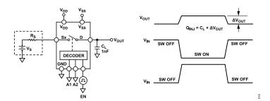
Figure 33. Charge Injection
