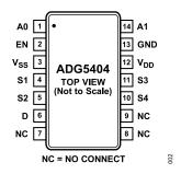
Figure 2. TSSOP Pin Configuration
