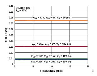
Figure 22. THD + N vs. Frequency, ±15 V Dual Supply
