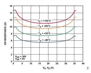
Figure 11.  $R_{ON}$  as a Function of  $V_D$  ( $V_S$ ) for Different Temperatures, 36 V Single Supply
