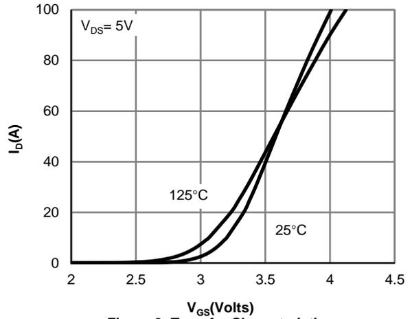
**Figure 2: Transfer Characteristics**
