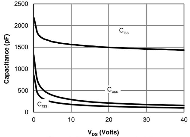
**Figure 8: Capacitance Characteristics**
