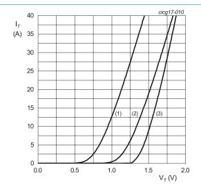
$V_o$  = 1.126 V;  $R_s$  = 0.0200 Ω (1)  $T_j$  = 150 °C; typical values (2)  $T_j$  = 150 °C; maximum values (3)  $T_j$  = 25 °C; maximum values
