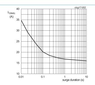
f = 50 Hz; T<sub>mb</sub> = 117 °C Fig. 2. RMS on-state current as a function of surge duration; maximum values
