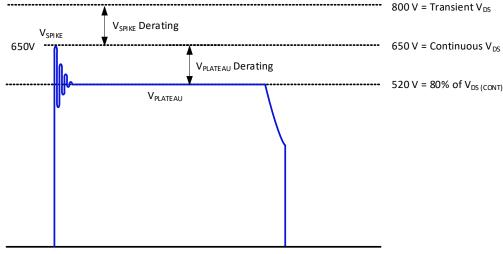
Fig. 28. QR flyback drain-to-source voltage stress diagram
