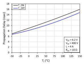
Fig. 14. Propagation delay ( $T_{ON}$  and  $T_{OFF}$ ) vs. junction temperature( $T_{II}$ )
