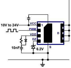
Fig. 18. Quick start-up circuit
