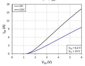
Fig. 5. Source-to-drain reverse conduction voltage
