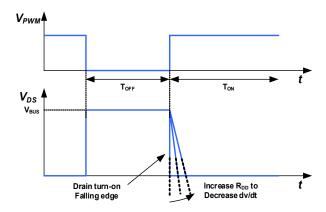
Fig. 23. Turn-on dV/dt slew rate control
