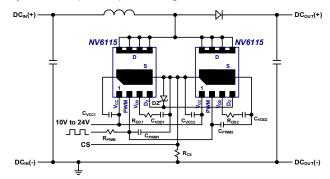
Fig. 25. Boost schematic using two parallel ICs
