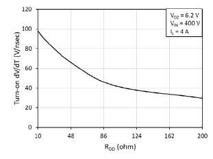
Fig. 15. Slew rate (dV/dt) vs. gate drive turn-on current set resistance ( $R_{\rm DD}$ ) at T = 25 °C
