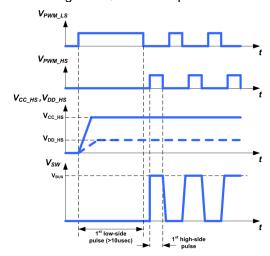
Fig. 19. LLC half-bridge start-up timing diagram
