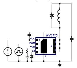
Fig. 1. Inductive switching circuit
