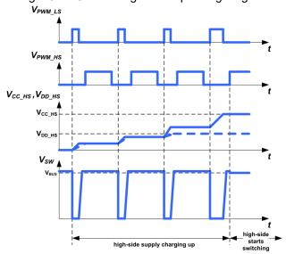
Fig. 20. ACF half-bridge start-up timing diagram
