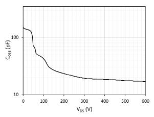
Fig. 9. Output capacitance  $(C_{OSS})$  vs. drain-to-source voltage  $(V_{DS})$
