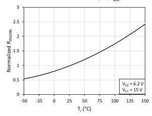
Fig. 8. Normalized on-resistance  $(R_{DS(ON)})$  vs. junction temperature  $(T_{,l})$
