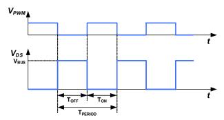
Fig. 21. Normal operating mode timing diagram
