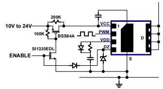
Fig. 22. Standby mode V<sub>CC</sub> cut-off circuit
