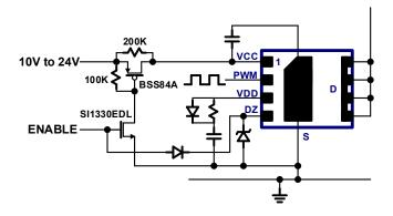
Fig. 22. Standby mode Vcc cut-off circuit
