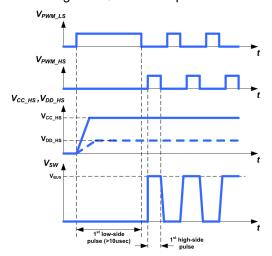
Fig. 19. LLC half-bridge start-up timing diagram
