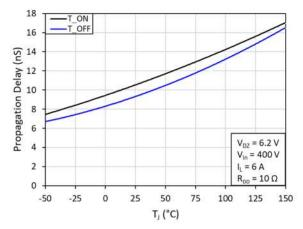
Fig. 14. Propagation delay ( $T_{ON}$  and  $T_{OFF}$ ) vs. junction temperature( $T_{IJ}$ )
