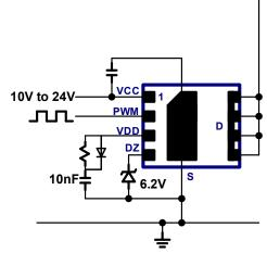
Fig. 18. Quick start-up circuit
