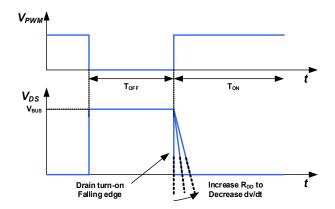
Fig. 23. Turn-on dV/dt slew rate control
