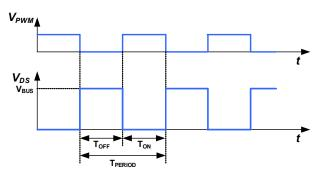
Fig. 21. Normal operating mode timing diagram
