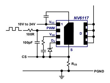
Fig. 24. Current sensing circuit
