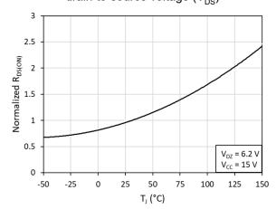
Fig. 8. Normalized on-resistance  $(R_{DS(ON)})$  vs. junction temperature  $(T_{,l})$
