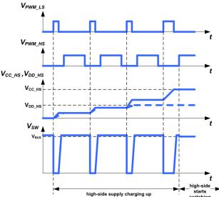
Fig. 20. ACF half-bridge start-up timing diagram
