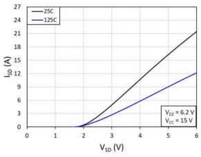
Fig. 5. Source-to-drain reverse conduction voltage
