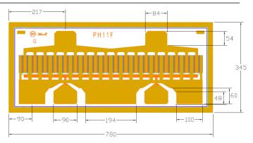
Chip Dimensions: 780 x 345 microns Chip Thickness: 100 microns
