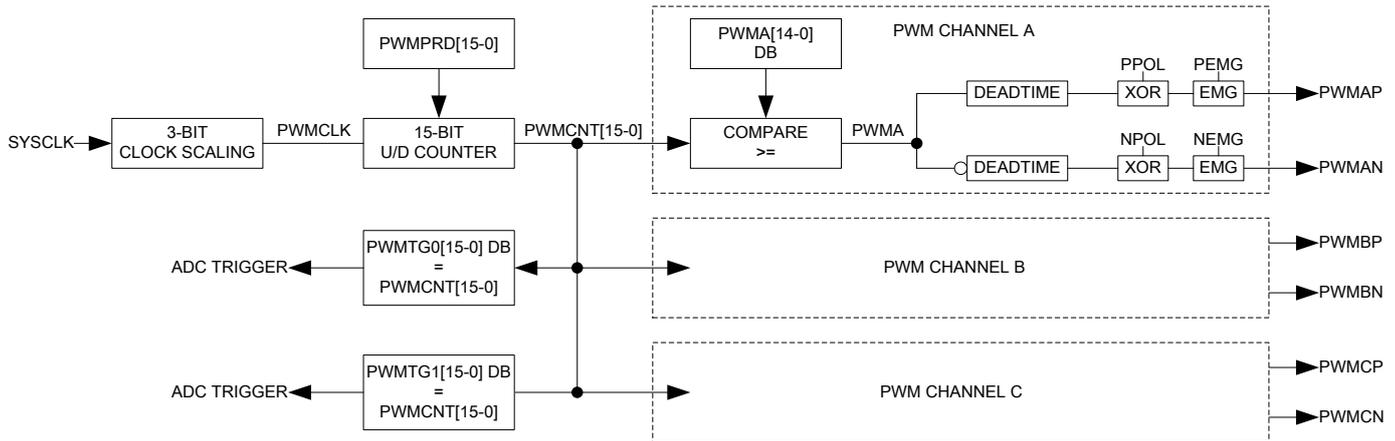
The period of the PWM frequency is defined by PWNPRD[14-0]. PWMPRD[15] is the enable control of the PWM and when read it represents up/down direction. A 15-bit Up/Down counter is used to provide the time base of the PWM channels. The operation of the PWM waveform is illustrated in the following timing diagram.
