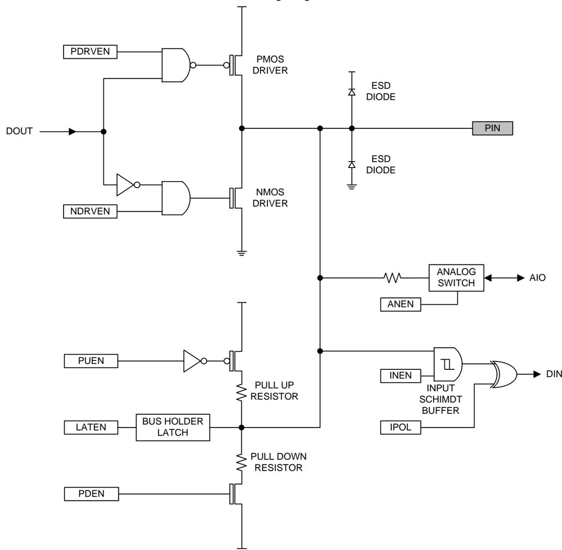
From the diagram, there are 7 control bits for the IOCFGPx.y register, and these registers are located at XFR 0xA040 – 0xA047 for P0.0 to P0.7, 0xA048 – 0xA04F for P1.0 to P1.7, 0xA060 – 0xA067 for P2.0 to P2.7, and 0xA068 – 0xA06F for P3.0 to P3.7. The definitions of IOCFGPx.y are described in the following table.
