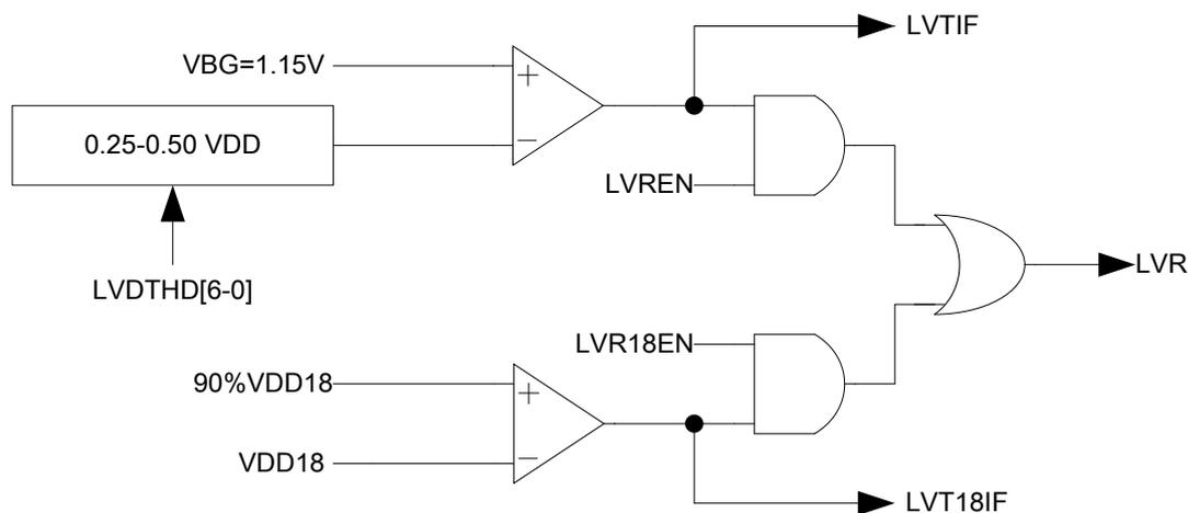
An enabled LVD circuit consumes about 100uA to 400uA depending on its VDD level. The LVDTHD[6-0] sets the compare threshold from 0.25VDD to 0.50VDD against the internal band-gap reference voltage of 1.15V. The detection threshold can be represented in the following equation when LVDTHV is the detection voltage.
