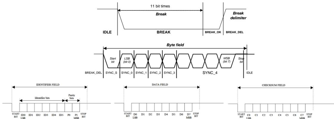
A LIN frame structure is shown and the frame time matches the number of bits sent and has a fixed timing.
