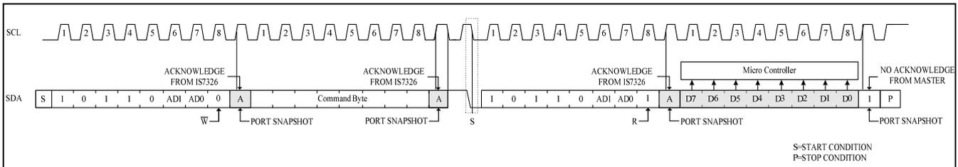
**Figure 6** Reading I/O Ports of IS31IO7326
