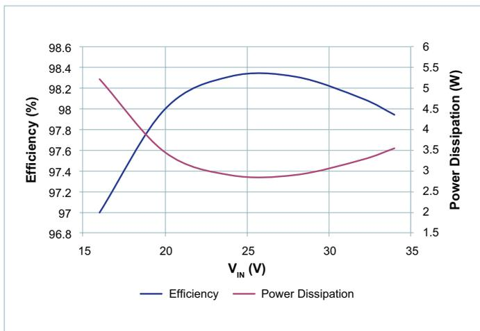
Figure 14 — 28V<sub>OUT</sub> Efficiency and Power Dissipation at 6A over Input Voltage Range
