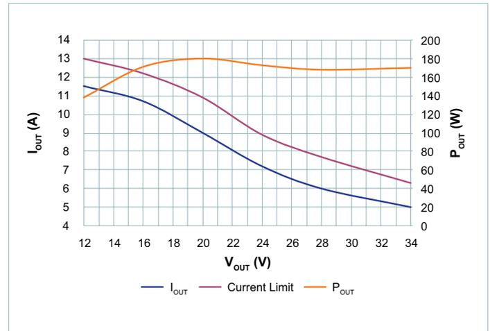
Figure 15 — Power and current output at 34V<sub>IN</sub>
