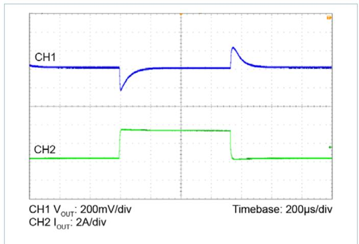
Figure 5 — 24V<sub>IN</sub> to 24V<sub>OUT</sub>,  $C_{OUT} = 8 \times 10\mu\text{F}$  Ceramic
