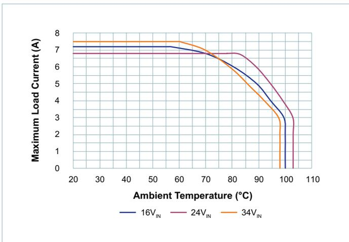
Figure 19 — Thermal de-rating @  $V_{OUT} = 24V$
