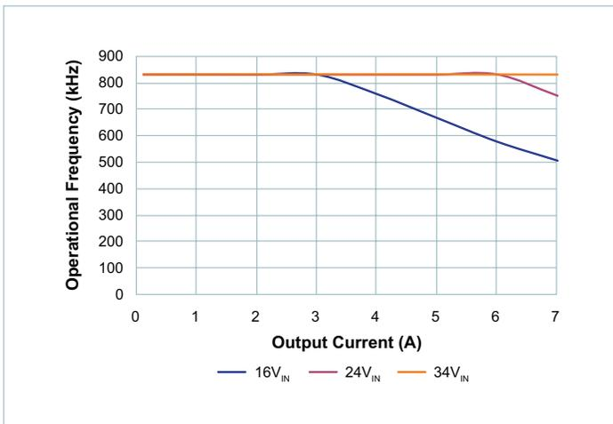
Figure 8 — Switching Frequency vs. Output Current @ 24V<sub>OUT</sub>
