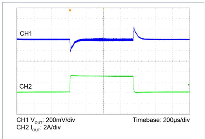
Figure 6 — 16V<sub>IN</sub> to 28V<sub>OUT</sub>,  $C_{OUT} = 8 \times 10\mu\text{F}$  Ceramic
