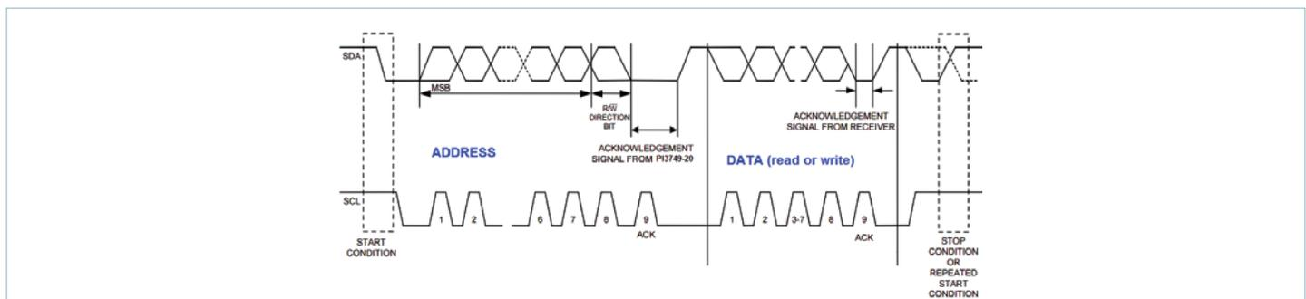
**Figure 28** — Data transfer on the I<sup>2</sup>C bus
