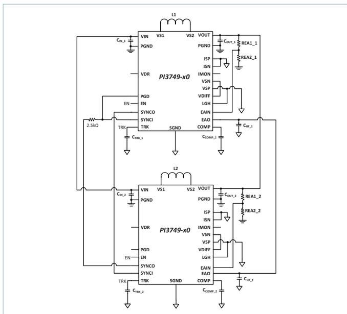
Figure 27 — PI3749-x0 parallel operation
