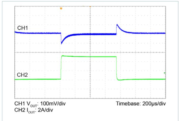
Figure 4 — 34V<sub>IN</sub> to 12V<sub>OUT</sub>,  $C_{OUT} = 8 \times 10\mu\text{F}$  Ceramic
