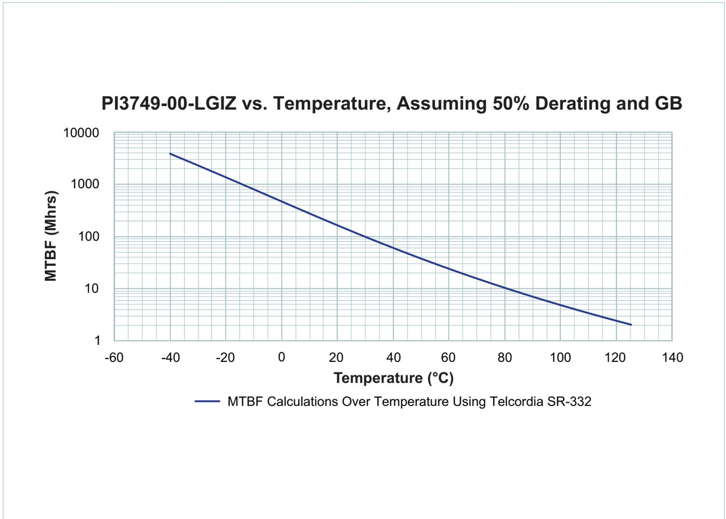
Figure 23 — PI3749-x0 calculated MTBF Telcordia SR-332 GB
