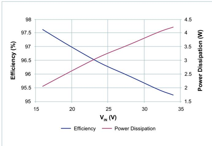
Figure 12 — 12V<sub>OUT</sub> Efficiency and Power Dissipation at 7A over Input Voltage Range
