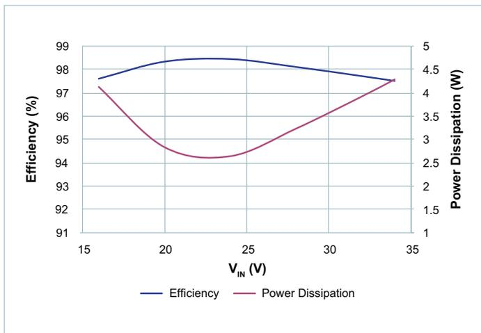
Figure 13 — 24V<sub>OUT</sub> Efficiency and Power Dissipation at 7A over Input Voltage Range
