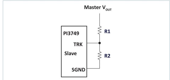
Figure 26 — Voltage divider connections for direct tracking
