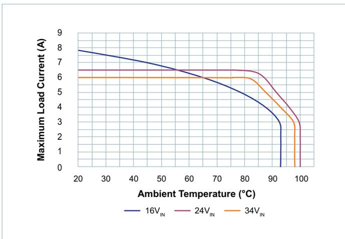
Figure 20 — Thermal de-rating @  $V_{OUT} = 28V$
