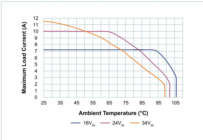
Figure 18 — Thermal de-rating @  $V_{OUT} = 12V$
