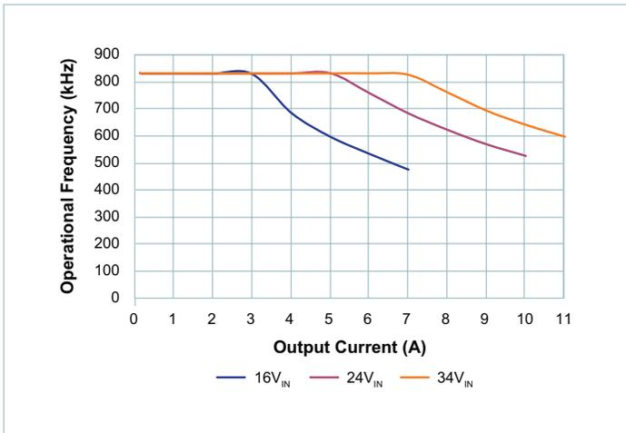
Figure 7 — Switching Frequency vs. Output Current @ 12V<sub>OUT</sub>
