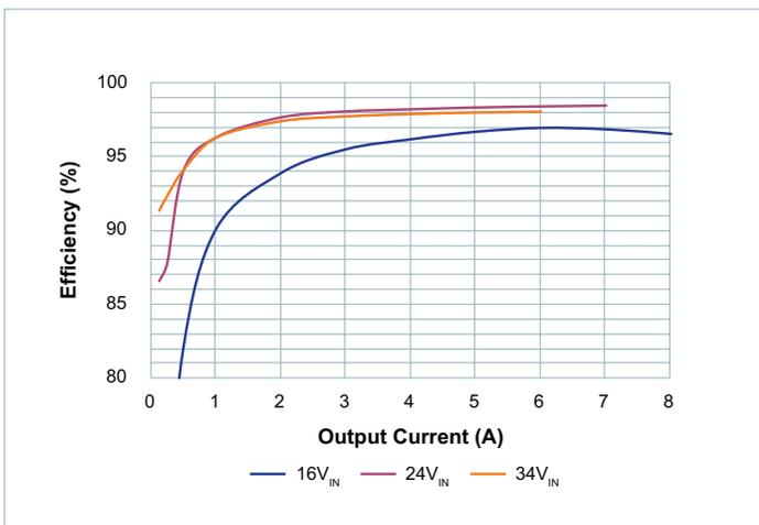
Figure 3 — 28V<sub>OUT</sub> Efficiency
