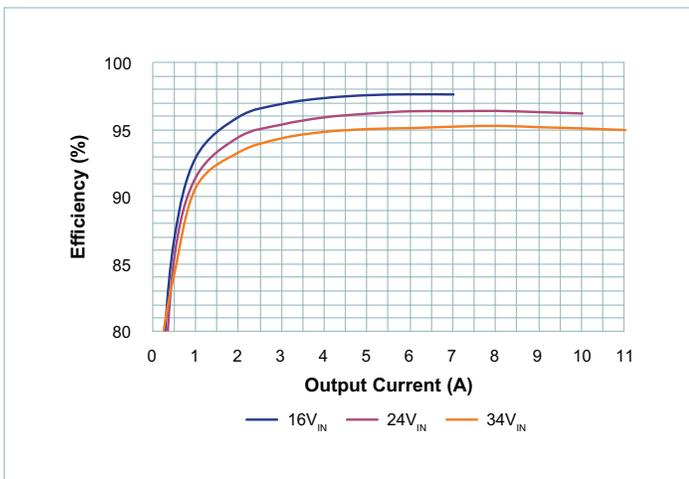
Figure 2 — 12V<sub>OUT</sub> Efficiency
