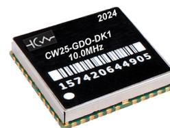
In addition to generating a phase aligned 1PPS output, the module generates three clock signals phase aligned to the 1PPS signal. Output clocks include one digitally synthesized clock output at frequencies from 150Hz to 80MHz and two low jitter 10MHz clock outputs generated from an integrated APLL block with options for 3.3V CMOS and/or differential LVPECL/LVDS signals at frequencies up to 700MHz
