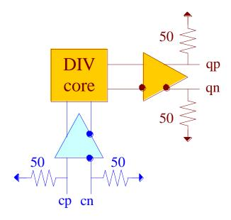
Fig. 1. Functional Block Diagram
