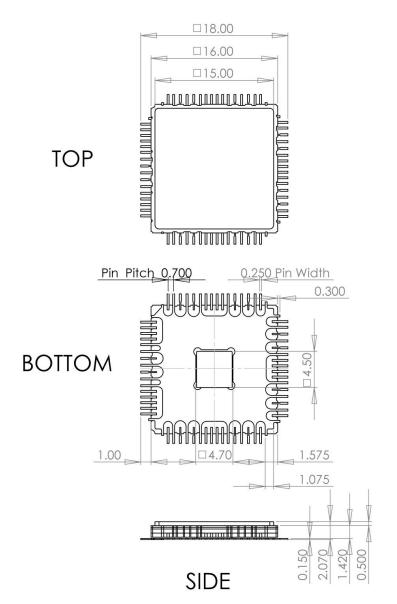
Fig. 6. CQFP 64-Pin Package Drawing (All Dimensions in mm)
